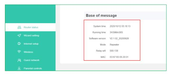
Note: If you use the universal relay mode (Client+AP) mode, after the relay is completed, the IP of the router is issued by the superior. At this time, if you want to login to the management interface of CR300, you need to set a static IP on the computer. The operation is as follows:
