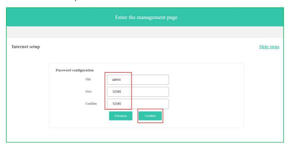
5. Wait about 10 seconds to complete the configuration. If you connect to the secondary router settings via wireless connection, you need to reconnect the modified wireless name.
