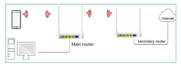
Please note: The secondary router does not need to be connected to the WAN port network cable.
