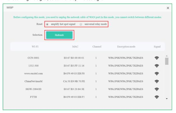
If the upper-level wireless signal has a wireless password, you need to enter the wireless password of the upper-level router, and then click "Connect", the router will restart automatically, wait for about 1 minute to complete the restart;
