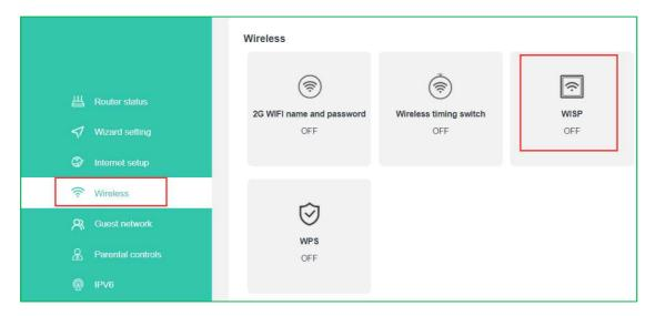
3.Turn on the WISP, select the relay mode "Amplified hotspot signal (WISP)" or "Universal relay mode (Client+AP)", and then click the refresh icon behind the wireless network selection.
